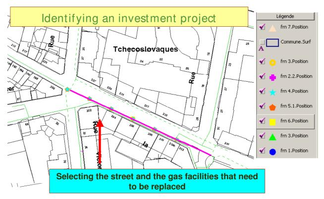
Having selected the pipelines in question, the application automatically identifies all the facilities that can be included in the study project, via map pointing around pipelines.
